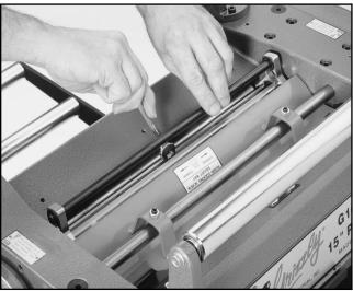
Figure 18. Tightening knives in cutterhead.
